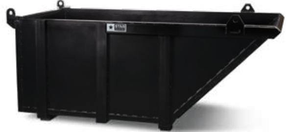
To dump the skip, the two forward slings are disconnected from the lifting eyes with the lifting line slack. The skip is then lifted with the rear slings still connected, effectively dumping the load from the sloped end.
