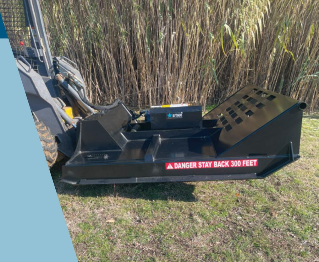
The Star Industries Skid-Steer Brush Cutter is the tough, all-terrain cutter perfect for clearing overgrowth on median strips, farm and ranch, parks and land clearing for development. The cutter is equipped with 3 versatile bi-directional blades powered by a high-torque motor and 100-hp Omni gearbox capable of powering through the toughest of terrains.
