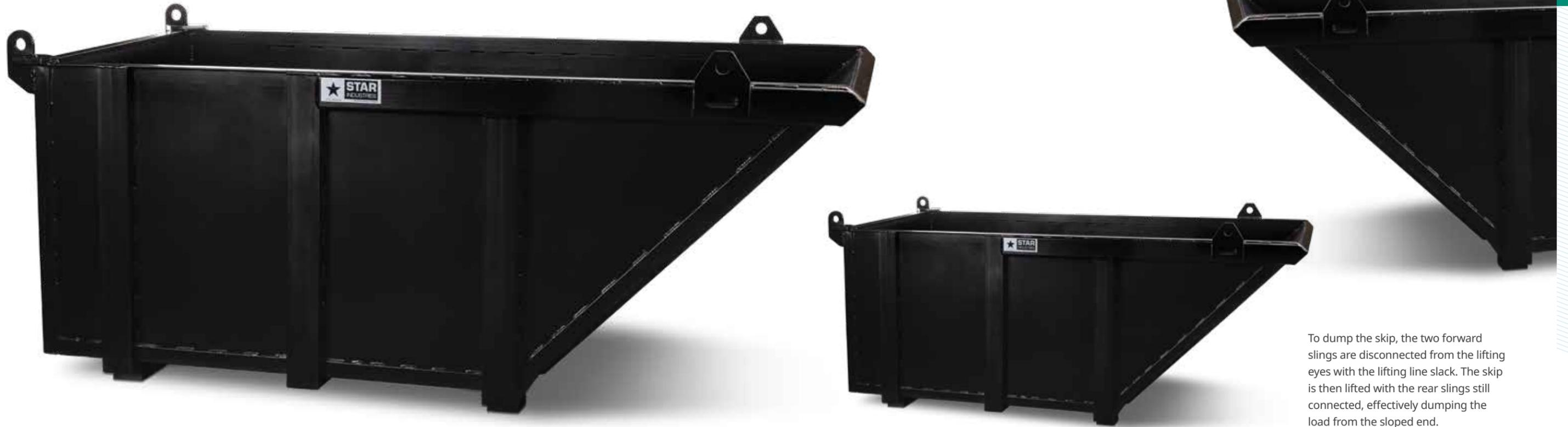
To dump the skip, the two forward slings are disconnected from the lifting eyes with the lifting line slack. The skip is then lifted with the rear slings still connected, effectively dumping the load from the sloped end.
