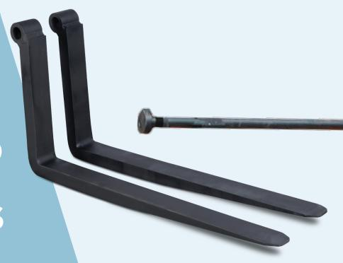
These shaft-mounted forks suit all pin-type carriages for telehandlers and rough-terrain forklifts, including models from: JLG, Cat, Skytrack, JCB, Genie/Terex, SkyJack, Pettibone, Xtreme, Gehl, Gradall, and Ingersoll Rand.
